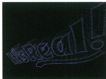
Fig. 2. (a) The 3D technique for generating chrome logos starts with a geometrical description of the object, shown here in wireframe. (b) The relationship between diffuse surface and specular highlight colors creates a flat and crude-looking chrome. (c) Geometry is partitioned and assigned contrasting diffuse colors to show off its volume better than light algorithms alone can do. (d) Ray tracing provides realistic reflections, though the geometry still reads rather flat. (e) Partitioning combined with adjusted ray tracing provides the highest realism. (Illustrations courtesy of Jens Scott © 1995.)
